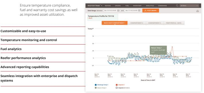
**ReeferTrak GlobalView** is an application for transportation companies that monitors and controls refrigerated assets. The ReeferTrak solution uses ORBCOMM devices and the ReeferTrak application to help ensure temperature compliance, fuel and warranty cost savings as well as improved asset utilization.
